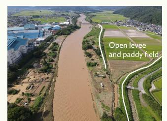
Figure 8.8: Example of an Open Levee and a Paddy Field
